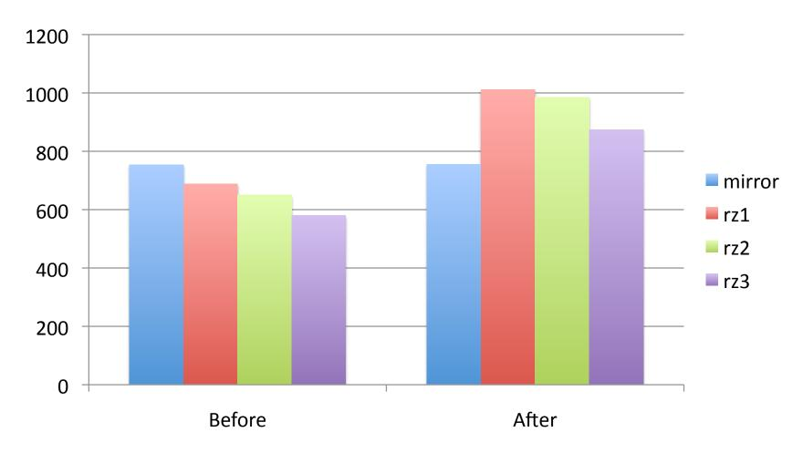
Sun Storage 7410, 48 x 1T 7200 RPM SATA (2009) Multi-threaded streaming write workload (MB/s)
